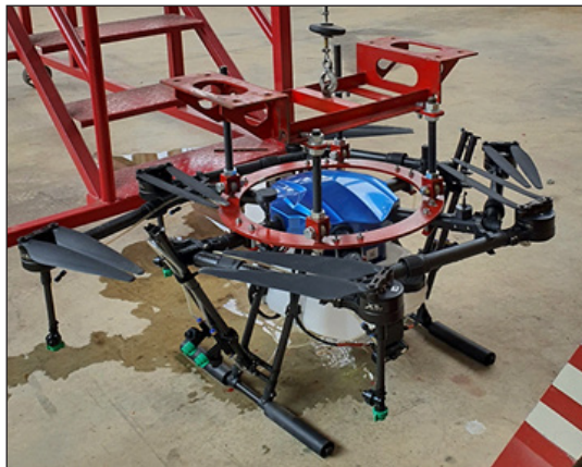
Figure 7. UAV is placed in a custom-designed mounting frame before mounting onto the testing rig
